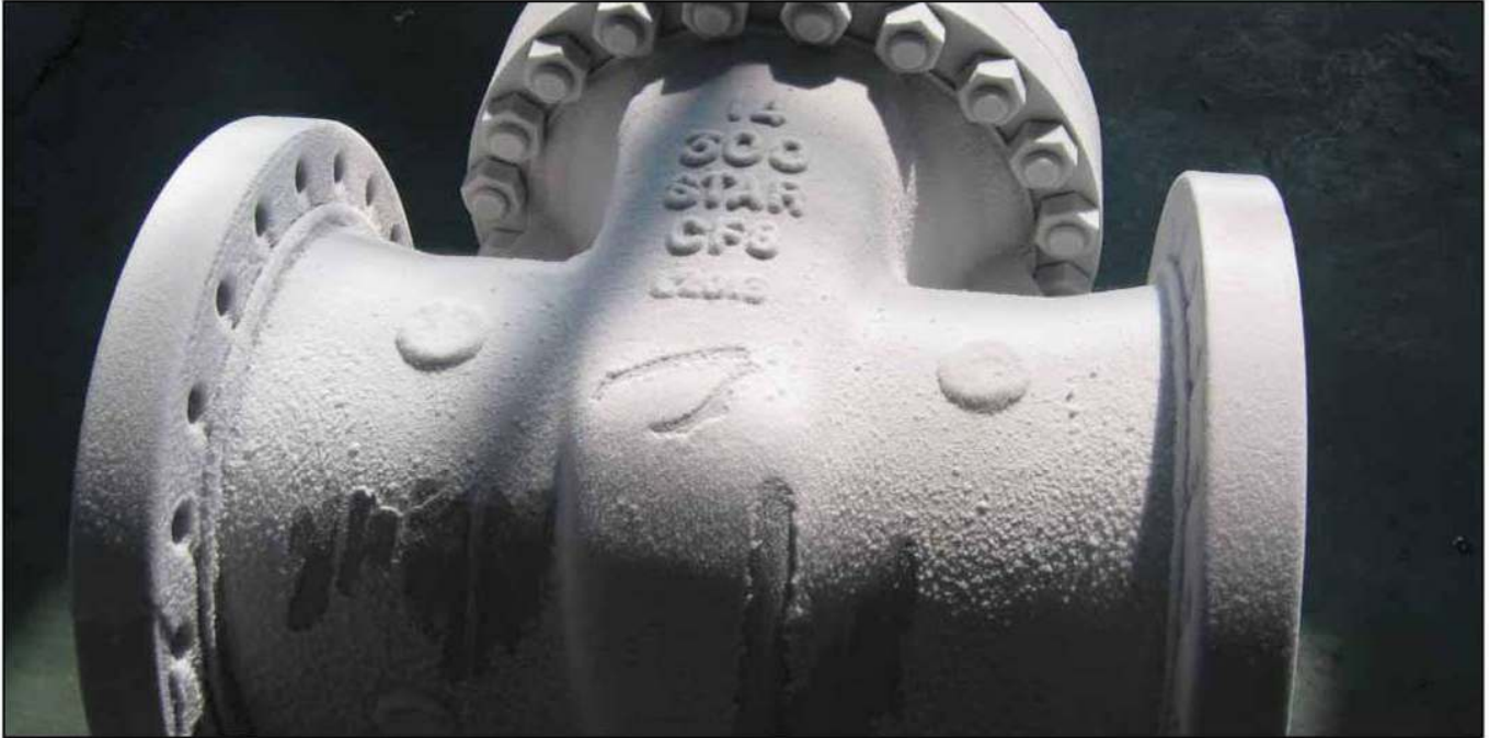
14" CLASS 300 CF8 gate valve, after cryogenic treatment.
