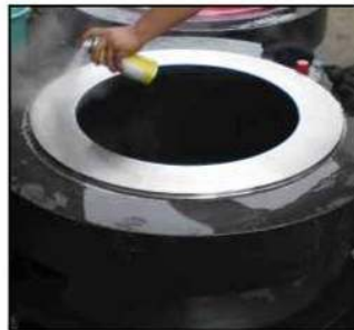
Dye penetrant test
