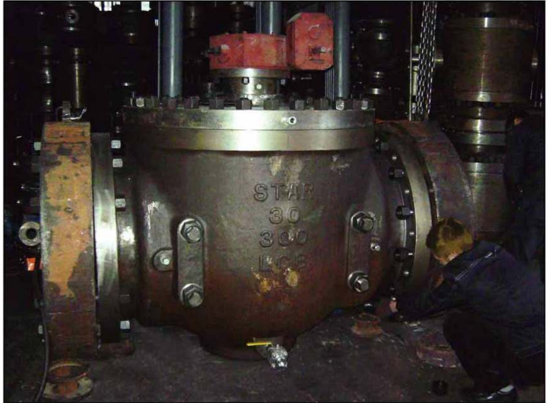
Testing of 30" 300# top entry ball valve
