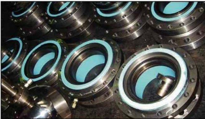
Assembly of trunnion mounted ball valve
