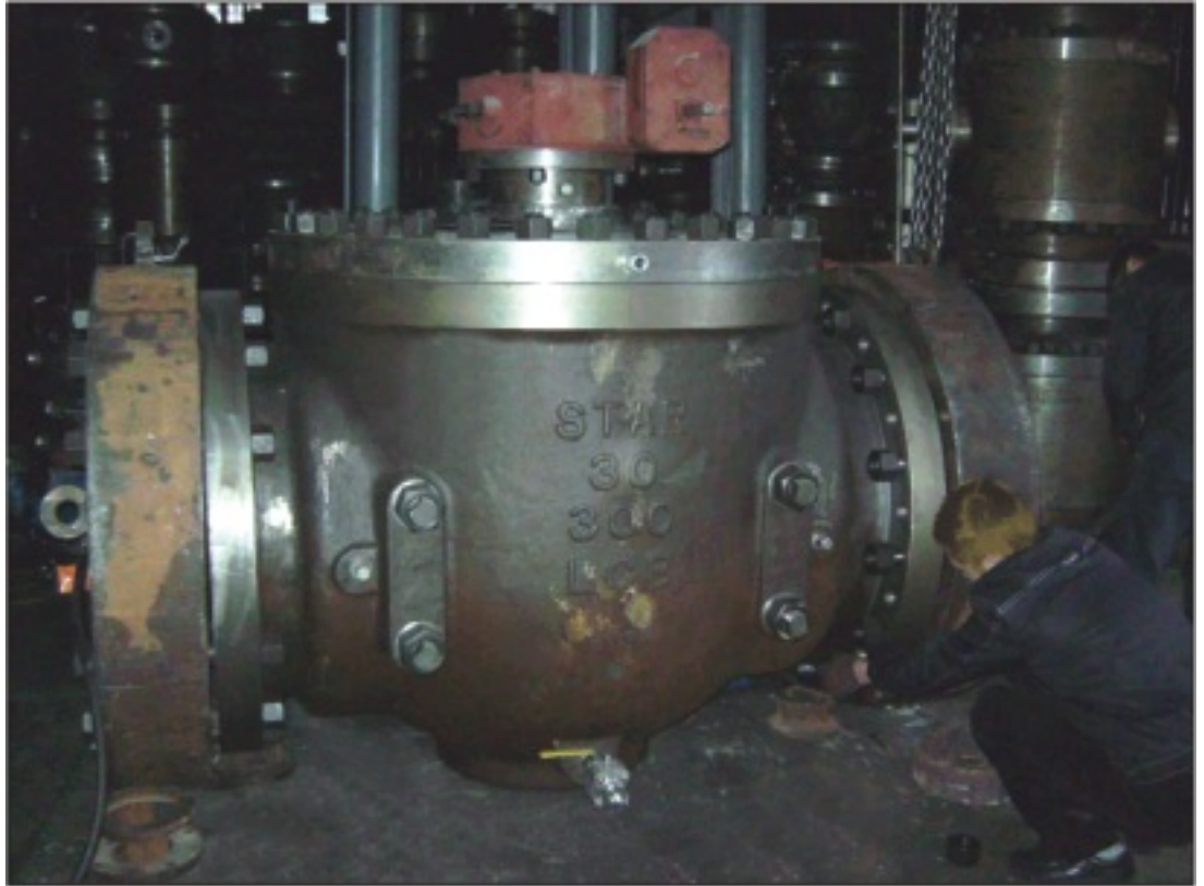
Testing of 30" 300# top entry ball valve
