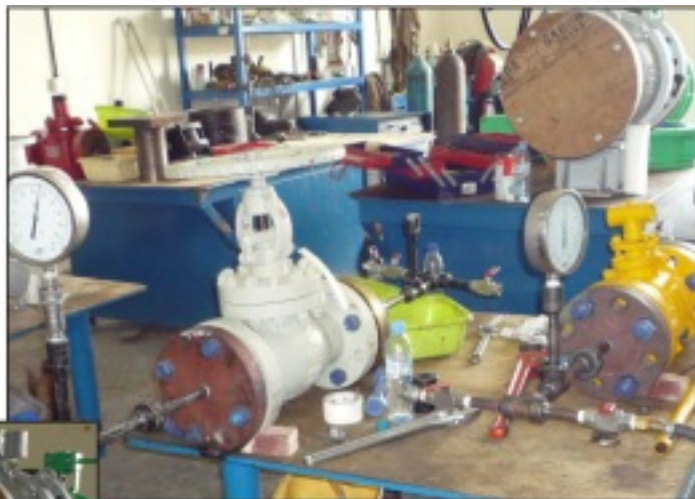
Globe valve under testing.
