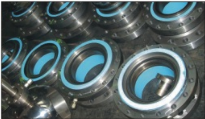
Assembly of trunnion mounted ball valve
