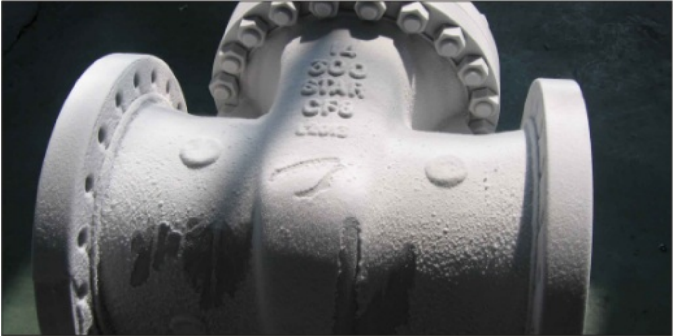
14" CLASS 300 CF8 gate valve, after cryogenic treatment.
